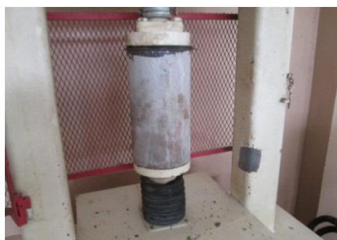
Figure 7 – Hydraulic press for the compression
