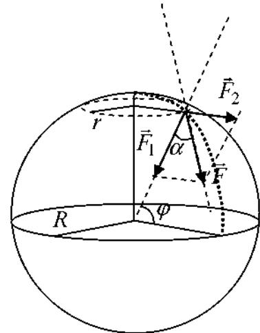
$$F_2 = ma_n = m\omega^2 r = m\omega^2 R \cos \varphi = m\left(\frac{2\pi}{T}\right)^2 R \cos \varphi$$
